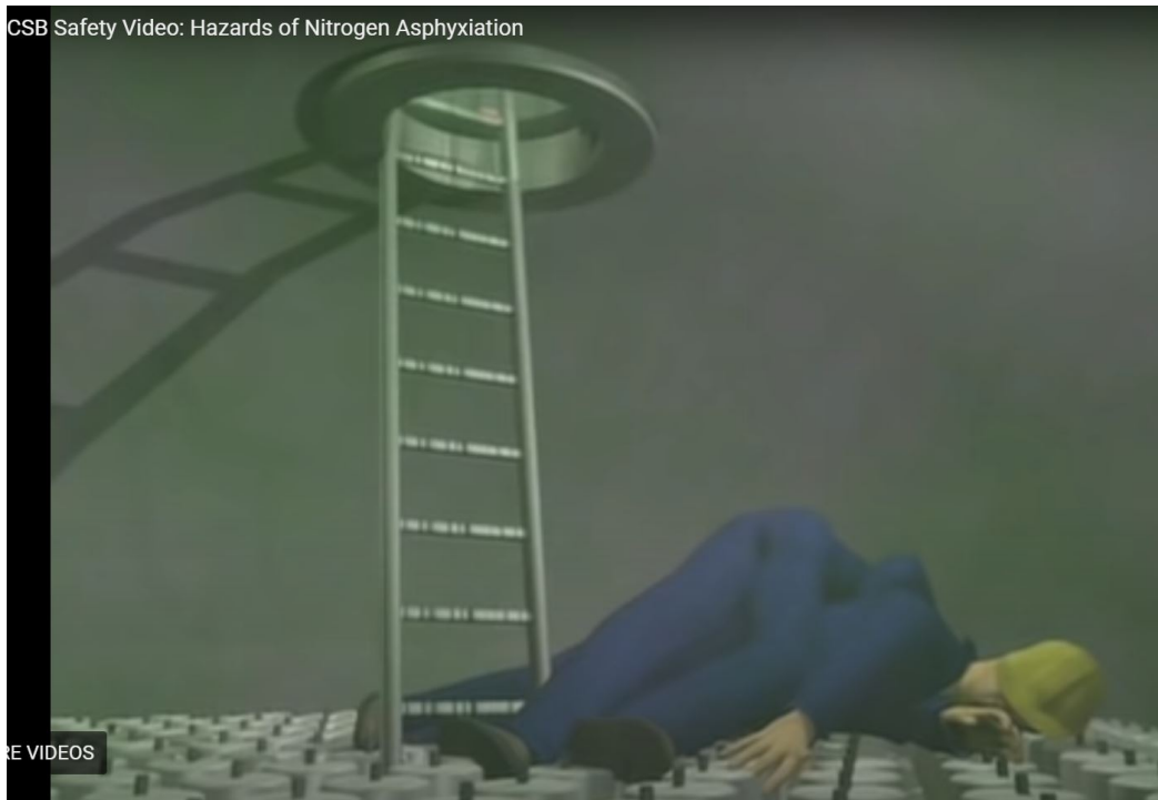
Figure 1. Collapse of two workers in a nitrogen atmosphere (from the CSB video).
